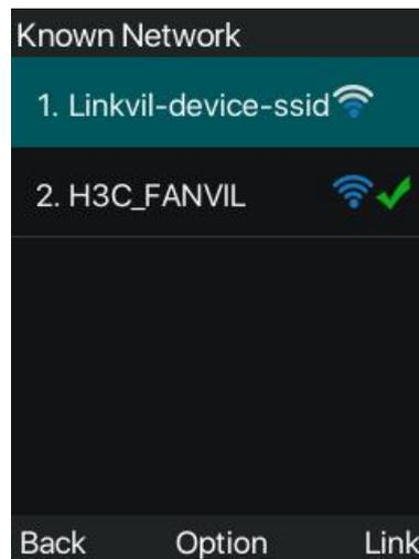
2) After the user connects to an AP, the user can enter [Menu] > [Advanced Settings] > [Share WiFi] on the device, turn on the WiFi sharing function, fill in the SSID, security mode, and password of the AP, and other devices that do not have any known network except the fixed SSID can automatically obtain this WiFi to realize the WiFi sharing function.
